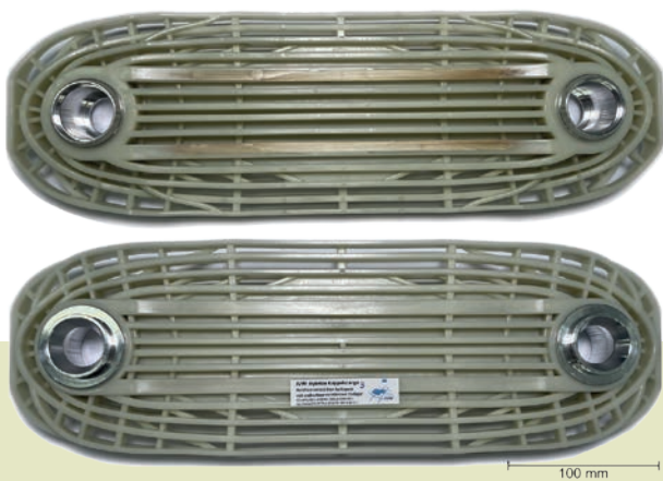
Front and rear side of the “Hybrid coupling rod” assembly with aluminum sleeves as bearing housing for ball studs
