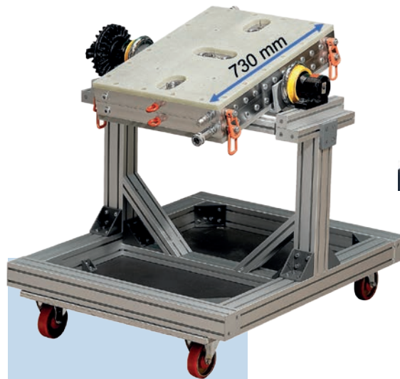
Stainless-steel injection tool with modular sensor inserts
