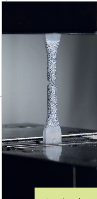
Approximated stress state in-between fibers by the use of a notched round specimen of neat polymer
