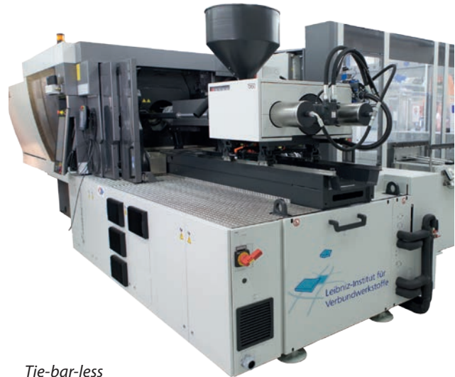
Tie-bar-less injection molding machine with automation cell
