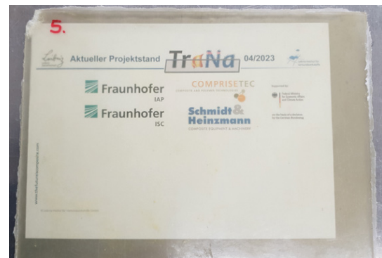
Translucent and flame retardant SMC plate with LDH filler material (paper with imprint behind SMC plate)
