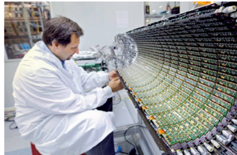
Stave Montage in Layer 2 Mounting of stave in layer 2
